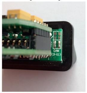
**Warning**: Please pay your attention to the fact that after you cross the CAN BUS to other pins, the pinout functionality will be also changed. That is if you cross the second CAN BUS and give an order to set voltage onto 11 pin of OBD2, then you will set the voltage to the pin where CAN Lo was crossed. Crossing of the second CAN BUS can be useful for diagnostics of some additional vehicle systems (ABS, multimedia and others) which can be located in various cars on different OBD2 pins.
