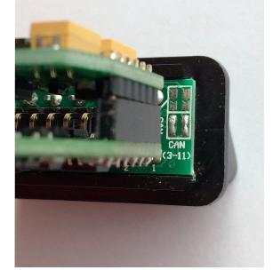
**Warning**: Please pay your attention to the fact that after you cross the CAN BUS to other pins, the pinout functionality will be also changed. That is if you cross the second CAN BUS and give an order to set voltage onto 11 pin of OBD2, then you will set the voltage to the pin where CAN Lo was crossed. Crossing of the second CAN BUS can be useful for diagnostics of some additional vehicle systems (ABS, multimedia and others) which can be located in various cars on different OBD2 pins.
