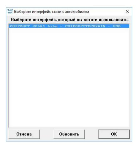
Taking into account that the CHIPSOFT J2534 Lite adapter does not have the integrated multiplexer to switch the K-Line pins automatically, work with all the ECUs is carried out on the main K-Line (7 pin of the OBDII socket). That is for ECU diagnostics which is using for example 12 pin of the OBDII socket, it is necessary to cross 12 pin of OBDII socket of the car to 7 pin of OBDII socket of the CHIPSOFT J2534 Lite adapter.
